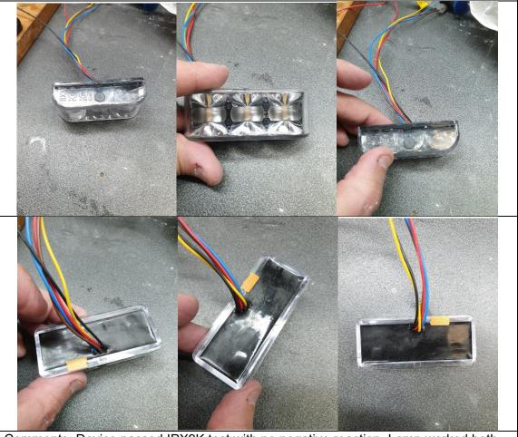
Comments: Device passed IPX9K test with no negative reaction. Lamp worked both at beginning of test cycle, during and after test cycle complete.
