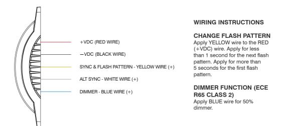
! WARNING ! - Unconnected wires MUST be sealed to prevent any water ingress.
