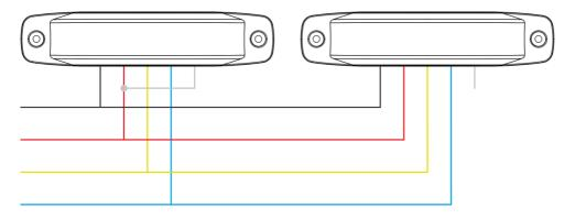
NOTE - With the power turned OFF, for Group 1, connect the WHITE wires to the RED(+) wire. For Group 2, leave the WHITE wires unconnected. The patterns will alternate when the power is turned ON.
