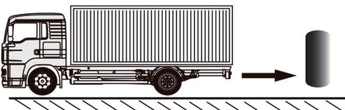
The sensors may not detect any sponge-like material obstacle as the ultrasonic wave was absorbed.
