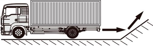
When the car approaches a smooth slope, the slope may not be detected.
