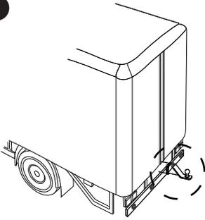
For example, if there is a tow bar, the back of truck and the system always detects it and sends false alarm.
