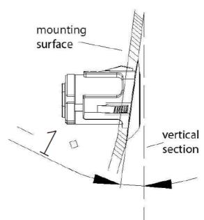
There are three kinds of (4°/8°/12°) sleeves to choose from. For example, for a location with a 50cm mounting height and -1°angle against vertical section (as shown in above picture). Then the computing method is:
